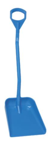
Robust hygiene shovel. The handle of this shovel is re-inforced with an inner aluminium tube. It is stepped in two places which helps to prevent back injuries. The neck joint has been strengthened in order to withstand heavy duty use. The short handle and small blade combination make it light weight and able to fit into smallish containers. Sometimes use as a large-scale dustpan.
